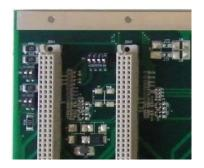
CAN Bus communication outputs + RS485 port to remote displays
