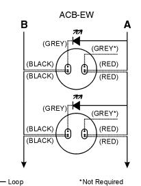
NOTE: Suitable waterproof crimps MUST be used between flying leads and loop cables.
