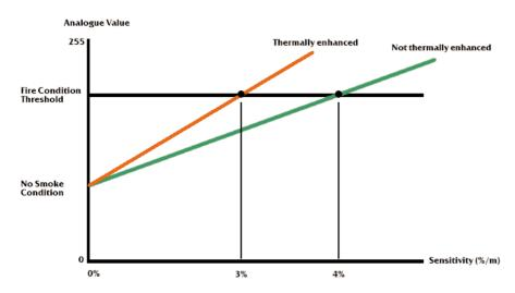
This graph shows how the ACA-E Multi-Sensor's photoelectric smoke sensitivity is enhanced when the temperature exceeds 40°C in Multi-Sensor Mode.
