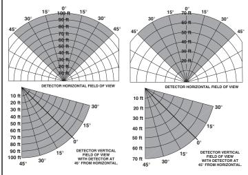
Field of View at Indicated Distance in Feet for **Hydrogen** at **Very High** Sensitivity (100 gm/min)
