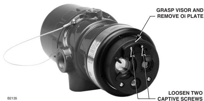
Figure 17—Oi Plate Removal
