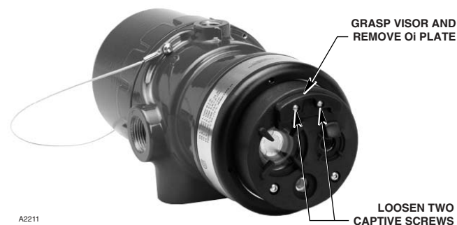
Figure 17—Oi Plate Removal
