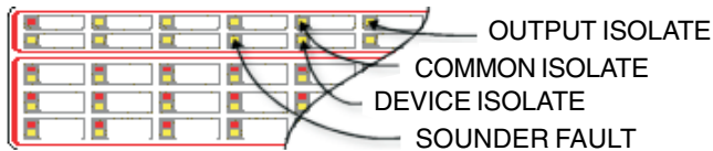
Figure 20 – Standard Control Panel Example Output Group Isolation
